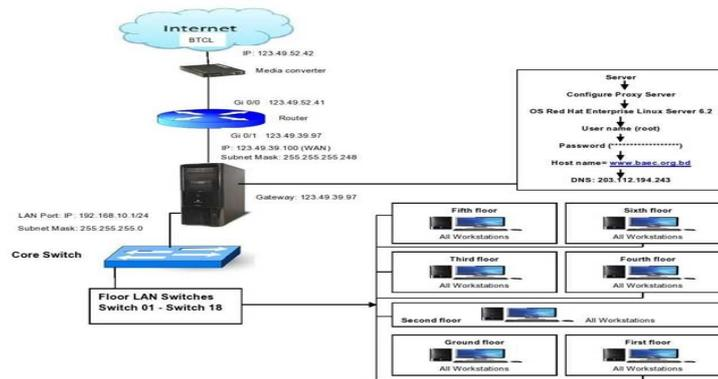
Figure 6: LAN Connection of BAEC Head Quarter.
